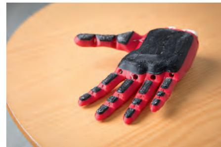
**The prosthetic (final model not shown) is made from a tough but flexible plastic. Shark-strength fishing wire runs through the fingers**
