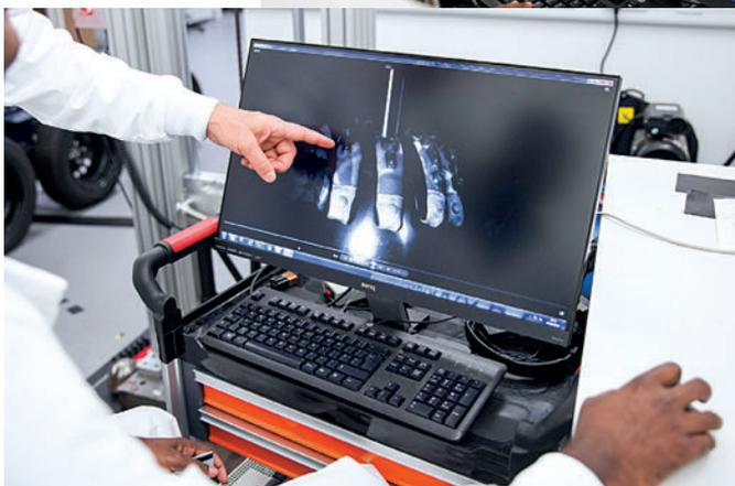
sophisticated tests in the Anti-Vehicle Underbelly Blast Injury Simulator. Here, compressed air is used to send blast waves through false and cadaver limbs (which are strictly approved and kept to an absolute minimum) that are laced with sensors to recreate the exact forces of blast impacts.
