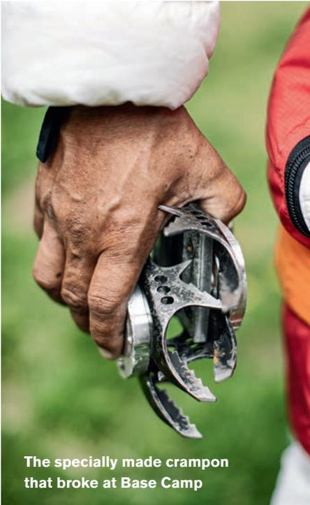
The specially made crampon that broke at Base Camp
